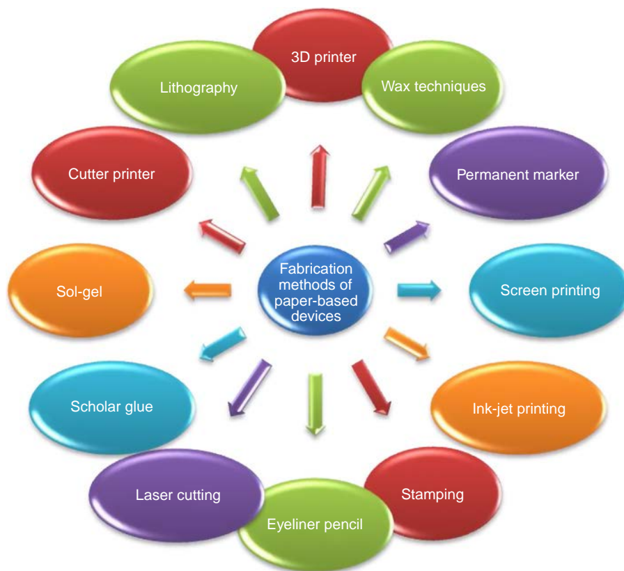
FIG. 25.1 Different fabrication methods involved in paper-based devices.
